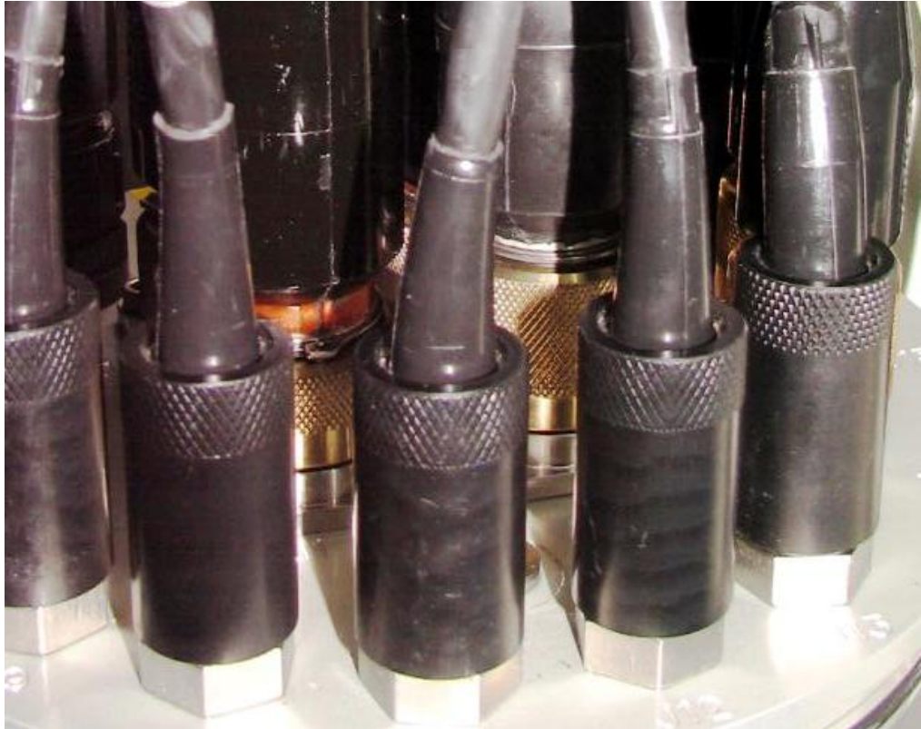
Figure 17 Crowded Can Head Inside PRM Showing Rubber Molded Connectors (Front Row) and Metal Shell Connectors (Back Row)
